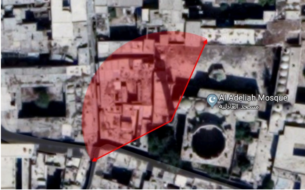
Danger area in case of the minaret collapse
